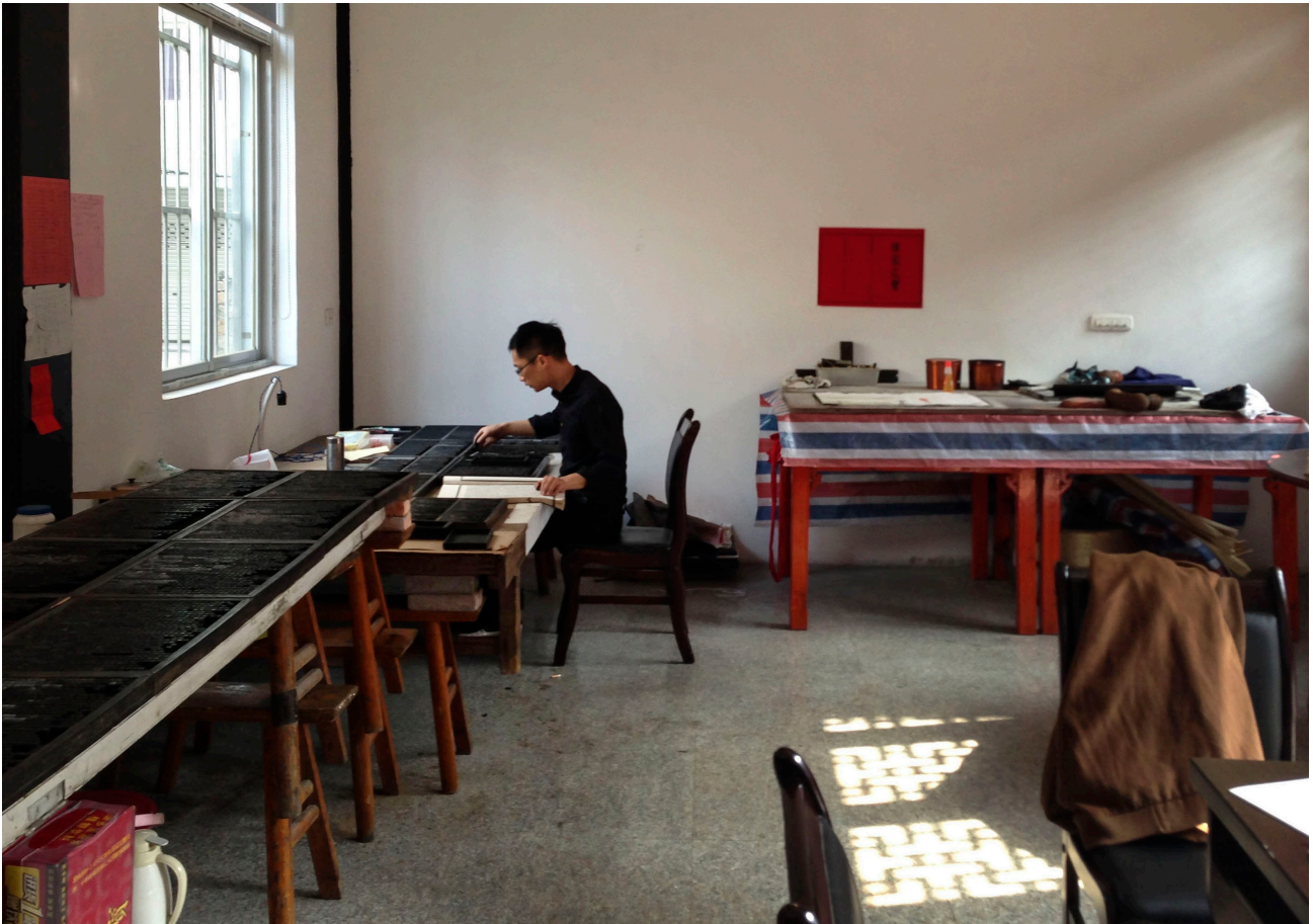
Photo 9 Work tables with all the types, up to 20,000 characters, are set up. The apprentices pick out the characters they need and put them together to compose the text in special frames that equal two pages. In order to find the right character fast they are placed in a special order depending on the character strokes and their position is memorised through a rhyme. The work requires a good memory, deft fingers, and a lot of walking back and forth between the tables and the different steps of printing.
