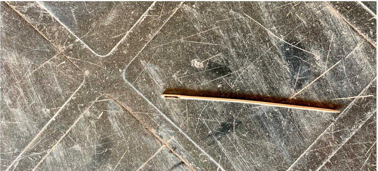
Photo 14 To repair plastic, the solution the Wichí men have found is sewing. Once heated, the needle – previously made of wood or bone, now made of metal and widely used by fishermen, but even more so by weavers – has become an essential tool for piercing broken parts. When it is a particularly resistant plastic, the awl is also used. The few mechanics in the region, more or less experienced, do not carry out this type of repair, which they consider to be a trivial DIY job that is not likely to last long, advising instead to buy a new fairing part. Thus, it is the people themselves who take care of this type of repair. distribution and avoid a second breakage. The reverse side of the set is just as important as the set itself.
