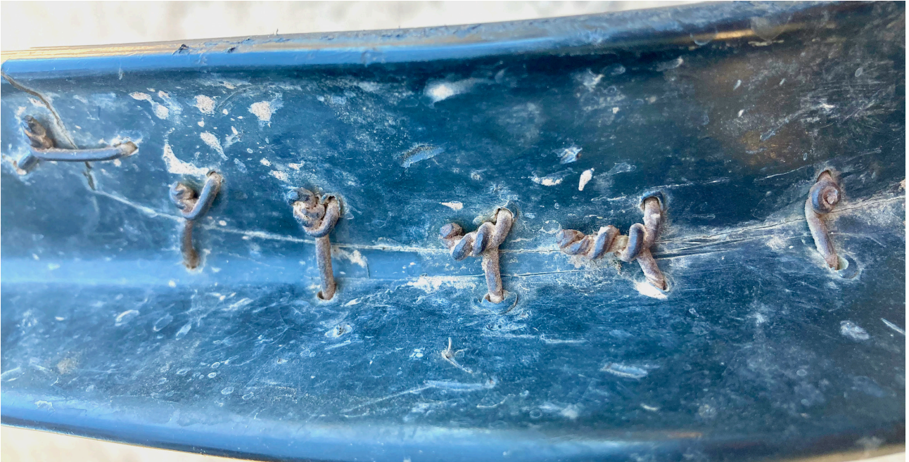
Photo 13 The reverse side of the seams, made in this case to repair the armrest of a chair, allow us to appreciate the finesse of the work done and the attention to detail. The wire has been cut cleanly to prevent clothes from snagging and the plastic has been punctured at regular intervals to optimise weight distribution and avoid a second breakage. The reverse side of the set is just as important as the set itself.
