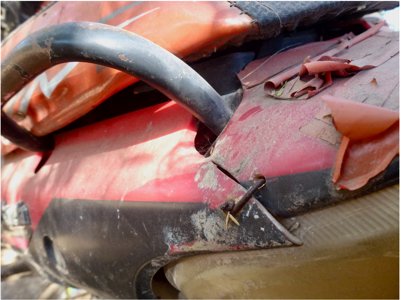
Photo 10 The parts no longer fit together, they have become damaged and when they broke, a piece was probably lost. But the wire keeps the fairing together. Indeed, once sewn together, the plastic pieces mend. The material loses its rigidity and more easily absorbs the shocks and vibrations to which the scooters are subjected every day on the region's mud tracks.
