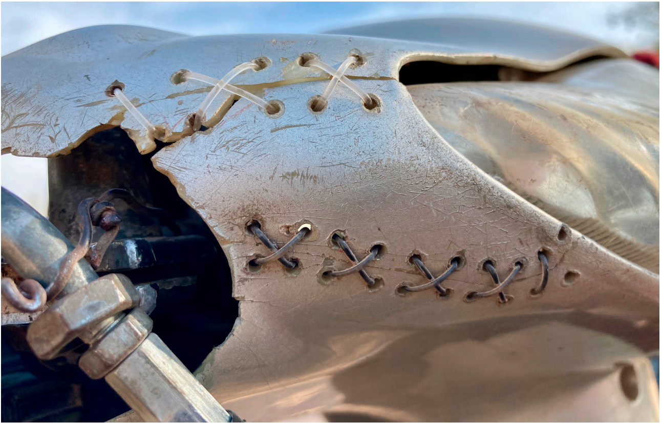
Photo 15 The stitching done with the needle technique leaves an everlasting mark on the fairing. Like so many scars, especially when it is a 'catch stitch', they recall the blows received and keep the memory of accidents, falls and shocks that punctuate the life of scooters and their riders. A slip on the sand, a blow from a tree branch or the backlash from a pit in a forest path are all events that can break the bumpers and plastic parts of two-wheelers. It is particularly interesting to note that two types of wire have been used. The fishing wire, which is very common, especially in the communities that live near the main rivers of the region, Pilcomayo and Bermejo. And the iron wire that characterizes the landscape of the contemporary Chaco, crossed by hundreds of thousands of fences that prevent access to recently deforested fields.
