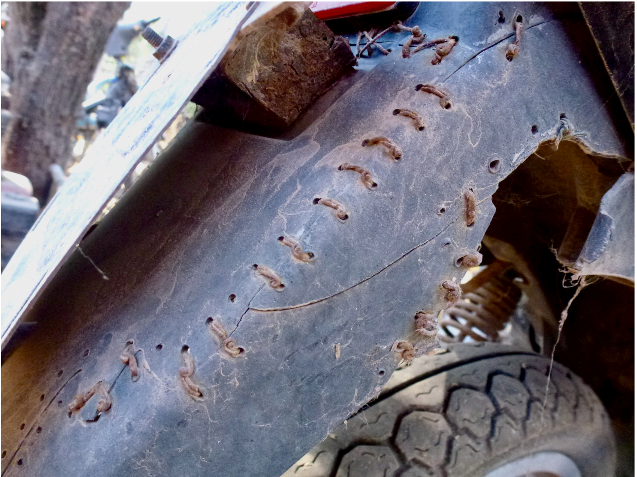
Photo 17 Without the seams, this mudguard would no longer hold together and it would have long since been abandoned in a dump. Bits and pieces are now lost forever, new fissures threaten the whole structure and points of the scar, now rusted and therefore less strong, have blown out. Despite this, the parts remain together and the integrity of the mudguard is maintained. Also interesting in this photo is the piece of wood that acts as a support for the number plate. The original one probably broke, so the owner managed to repair it with a more suitable material that is easier to find in the surrounding environment.
